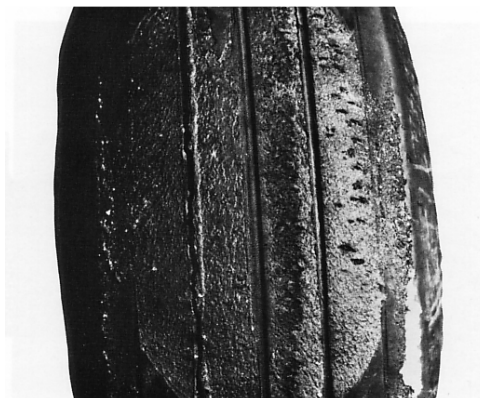
Tread Rubber Reversion An oval-shaped area in the tread similar to a skid, but where rubber shows burning due to hydroplaning during landing. Usually caused by wet or ice-covered runways. Remove if balance is affected.
