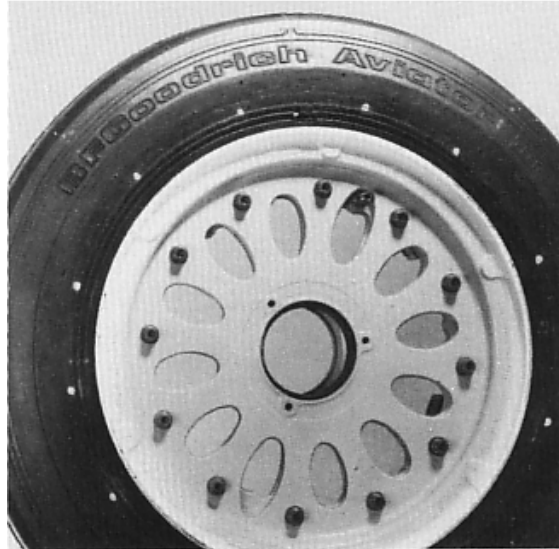
Typical tire vent markings.
