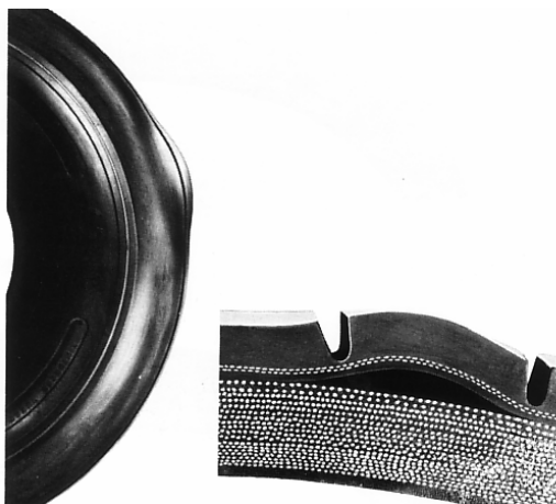
Tread Separation A rather large area of separation or void between components in the tread area due to loss of adhesion. Usually caused by excessive loads or flex heating from underinflation. Remove immediately.
