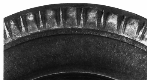
Ozone or Weather Checking/Cracking Random pattern of shallow sidewall cracks. Usually caused by age deterioration, prolonged exposure to weather or improper storage. Remove if fabric is visible.
