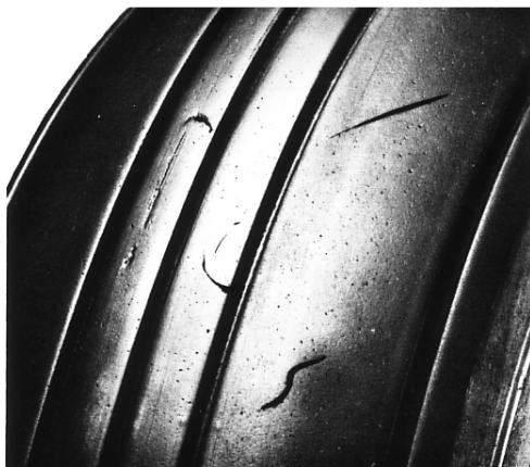
Cuts Penetration by a foreign object. Removal criteria: 1. Any cuts into the carcass ply. 2. Cuts extending more than half of the width of a rib and being deeper than 50% of the remaining groove depth.
