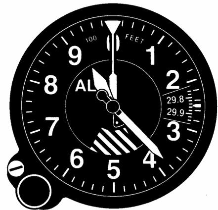
The newer style three-pointer sensitive altimeter uses a different pointer and a striped symbol that is visible below about 15,000 ft. as aids to make reading the altimeter easier.
